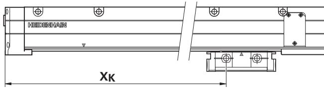
$$K [\mu\text{m}] = X_K [\text{m}] \cdot L_K [\mu\text{m}/\text{m}]$$
