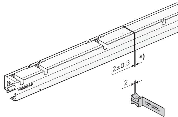
Slide the scale-tape housing **MG** onto the housing end section. Mind the gap!
