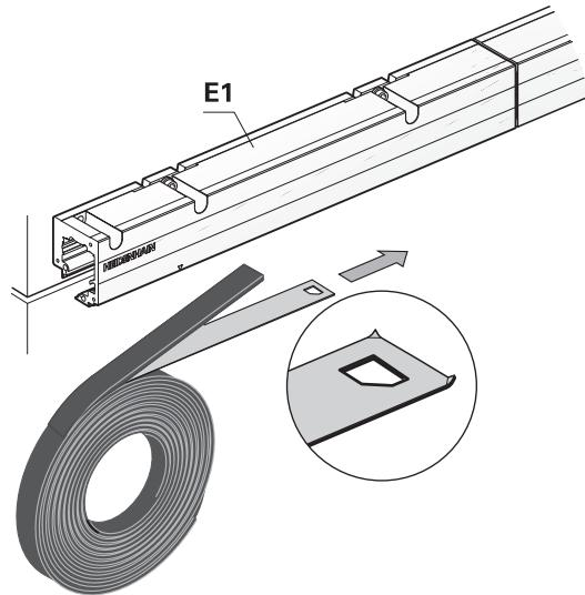
Insert the scale tape puller **EW**, hook in the scale tape and pull in.
