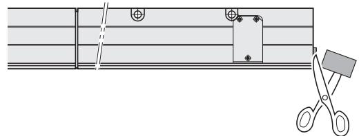
Using the slider **S**, orient the sealing lips outward over the entire length, making sure they protrude 1 mm.
