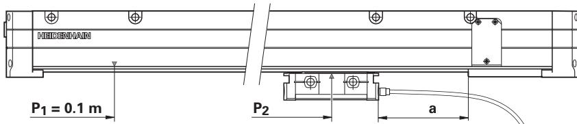
$$V [\mu\text{m}] = (P [\text{m}] - 0.033 \text{ m}) \cdot V_K [\mu\text{m}/\text{m}]$$
