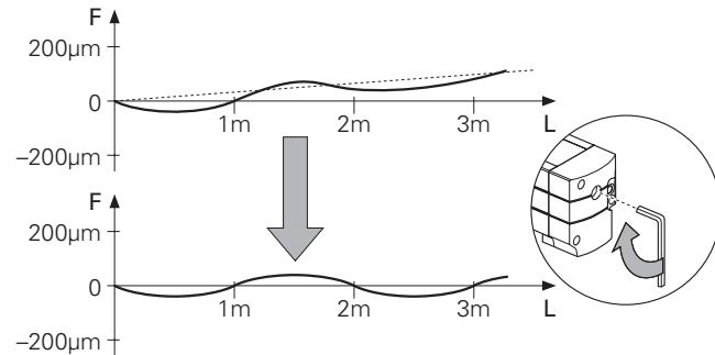
Set up a comparator system (such as a laser interferometer) in the workpiece plane and measure the machine.
