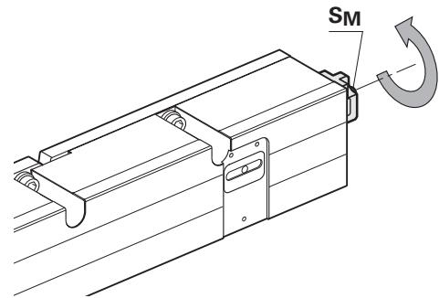
Then loosen the scale tape by 90° with the tape tensioning screw **S<sub>M</sub>**.
