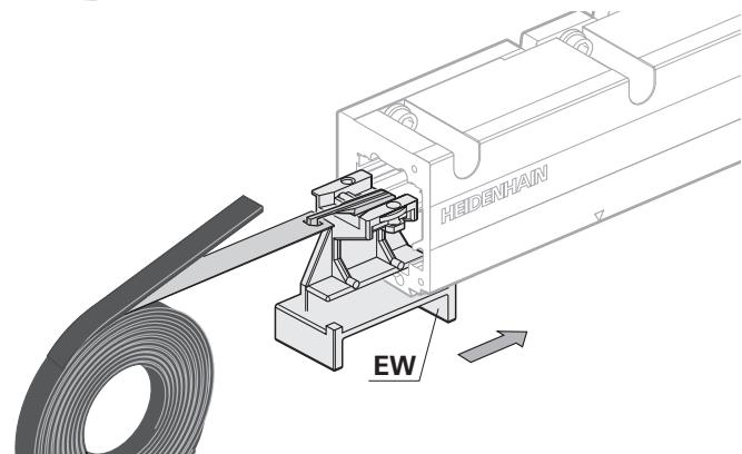
Unscrew the tape tensioning screw **SM** of the scale-tape tensioning device as far as possible and hook the scale tape in.
