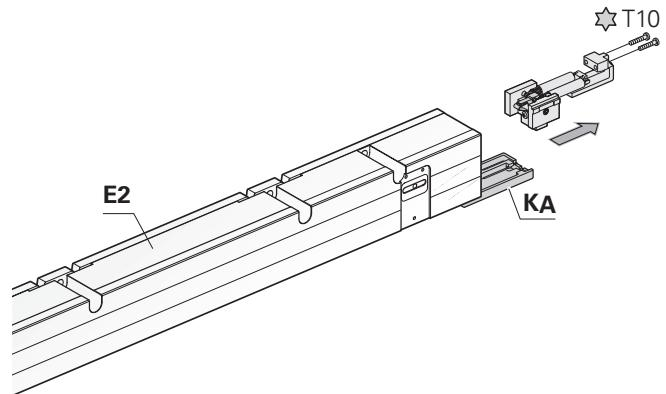
Slide housing end section **E2** onto the housing middle section, align and fasten.
