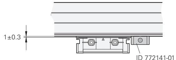
Check the mounting tolerances over the entire measuring length.
