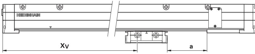
$$V [\mu\text{m}] = X_V [\text{m}] \cdot V_K [\mu\text{m}/\text{m}]$$
