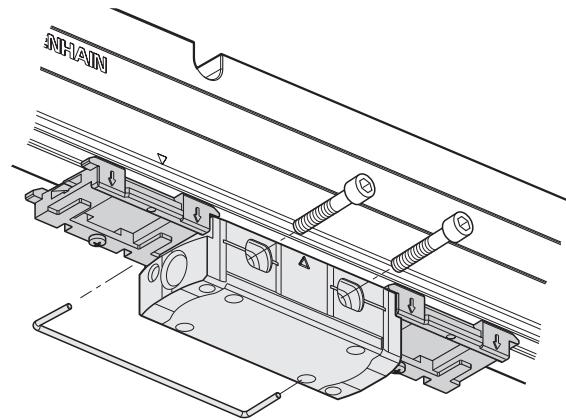
Set the scanning gap with the mounting gauge (ID 772141-01). Tighten the screws evenly. M6: **M<sub>d</sub>** = 8 Nm; M5: **M<sub>d</sub>** = 5 Nm. The scanning gap must be maintained over the entire measuring length.
