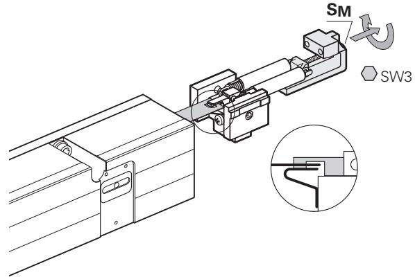
Slide in the scale tape with the tape tensioning device up to the stop and tighten the screws.
