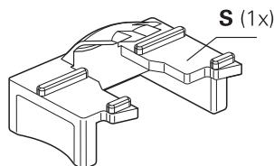
**Items supplied/Scale-tape housing, scanning unit**
