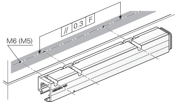
Screw on housing end section and align it to the machine guideway F.
