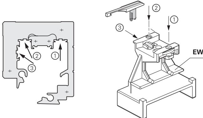
**Hook the bearing strips onto the catch such that beveled corners point upwards.**
