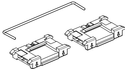
Click-in the shipping braces. If necessary, the screw **S** can be loosened or tightened.
