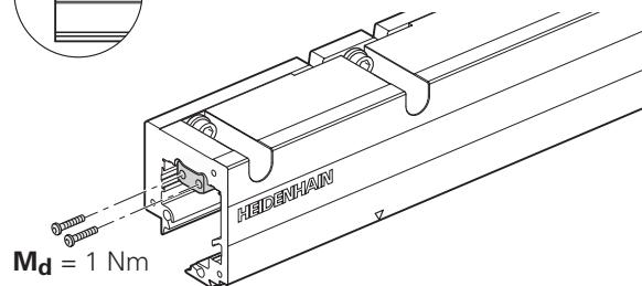
Tighten the tape tensioning screw **S<sub>M</sub>** just enough to remove any play from the tensioning device.
