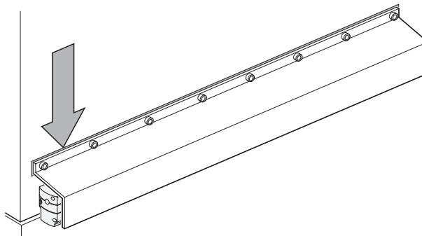
Choose a mounting attitude such that the maximum traverse range is within the measuring length ML of the encoder.
