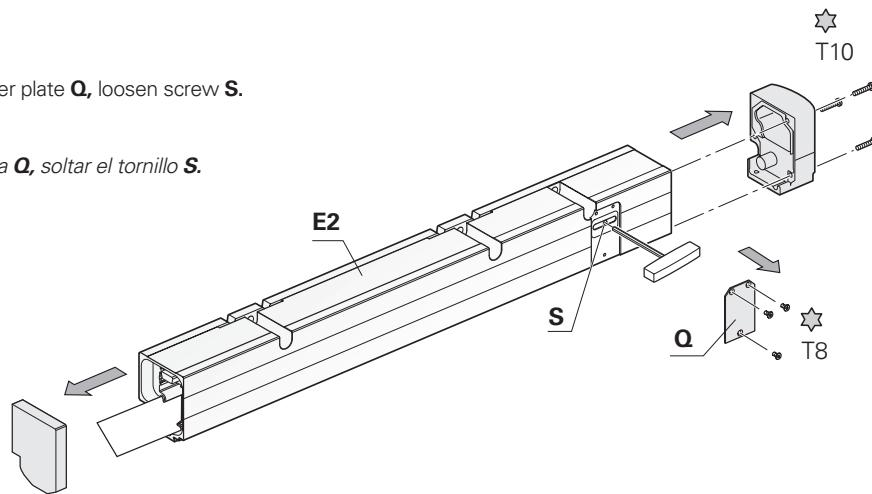
Detach the tensioning device from housing end section **E2**.
