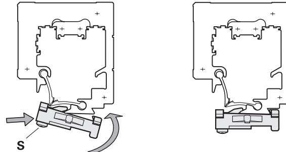
Carefully insert the scanning unit and, together with the first shipping brace, slide it into the housing until the second shipping brace can be clicked in.
