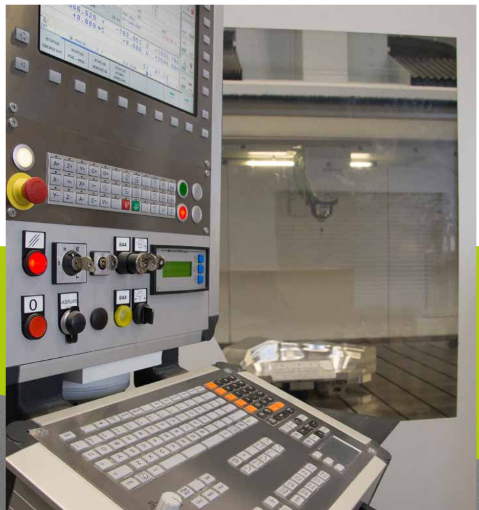
HEIDENHAIN iTNC 530 control: ideal functions for the manufacture of models and molds
