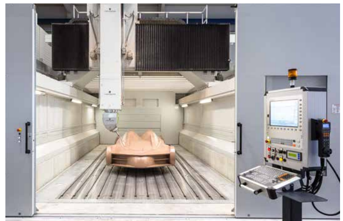
Model making on a large scale: the Zimmermann high-speed portal milling machines are customized to optimally meet the customer's requirements.
