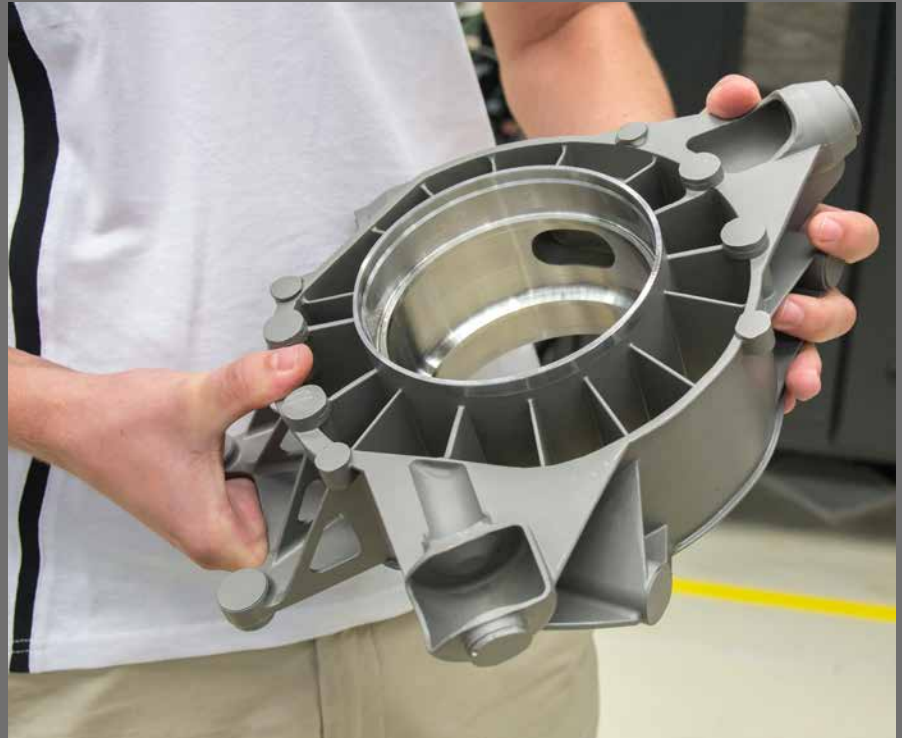
Upright for sports car: Machined with high accuracy using the HEIDENHAIN iTNC 530 control.
