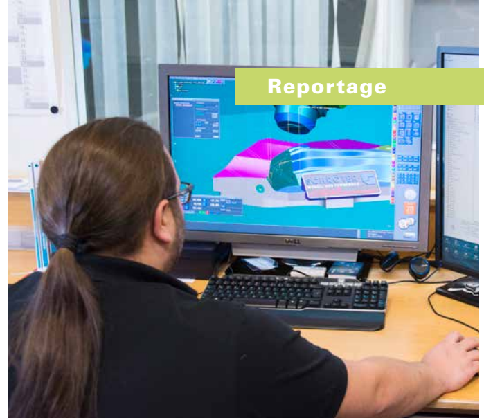
The same employee through all production stages: In the CAD/CAM system Martin Geisler prepares the model for production, generates the NC program, and then manufactures the model on the machine.
