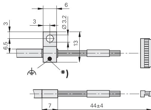
Mounting aid for inserting and removing the JST SHR-12V-S connector to avoid damage to the cable
