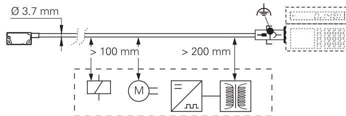
Permissible bending radii of connecting cable
