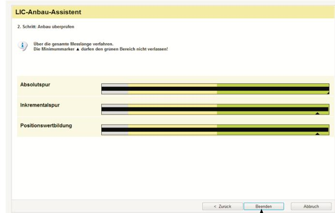
**Note:** If the green ranges are not reached or if strong signal oscillations occur over the entire measuring length, check the mounting tolerances and check for contamination.
