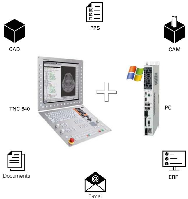
**Connected Machining** permits uniformly digital order management in networked manufacturing. You also profit from:
