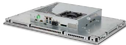
MC 366 with main computer installed on the back
